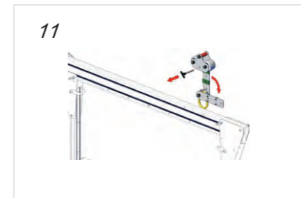
11 Remove pin. Open trolley and present to beam with plate rotated through 90°. Be careful not to allow plate to swing open uncontrolled.
