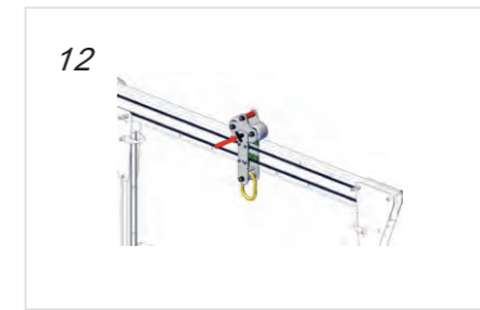
12 Close trolley plate encapsulating the beam and insert aircraft/ball-lock pin. Observe pin is properly engaged through holes.
