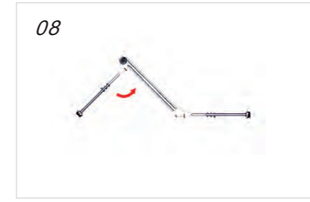
08 Scissor leg assembly until aircraft/ball-lock pin is adjacent to beam. Remove pin and continue scissor until stops engage beam and holes are aligned. Be careful not to trap hands between beam and cheek plates!
