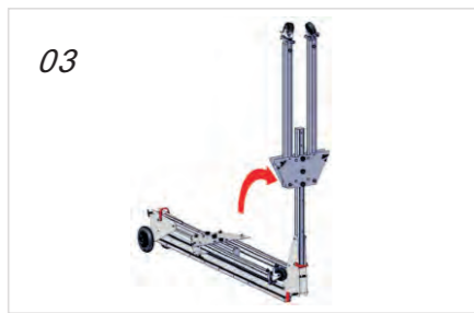
03 Rotate first leg assembly to a vertical position.
