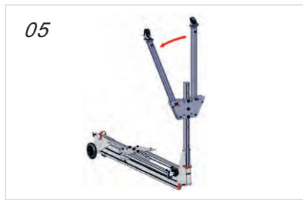
05 Open leg and insert aircraft/ball-lock pin into second hole securing the leg in its open position. Repeat for second leg.
